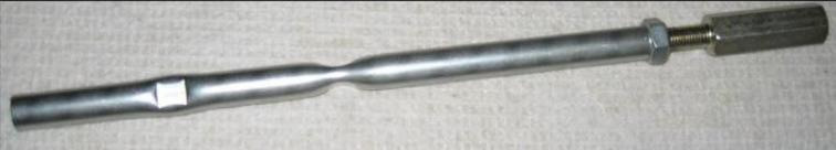
The tie rod extensions provided thread onto the ends of your current tie rods to extend them to match the width of the new suspension. It works
