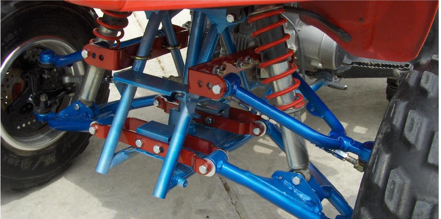
It's best to put all of the parts together before tightening anything. This is especially true for assembling the a-arms to the mount brackets. We've included large washers to be used between the brackets provided and the a-arm bushing to take up the space created by bolting on the outside of the stock frame mounts.
